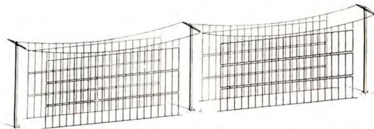
FIG. 4.—Vertical Wire Flat Transmitting Aerial and Reflector, 1924.
