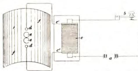
FIG. 1.—Spark Transmitter and Sheet Metal Reflector, 1896.
