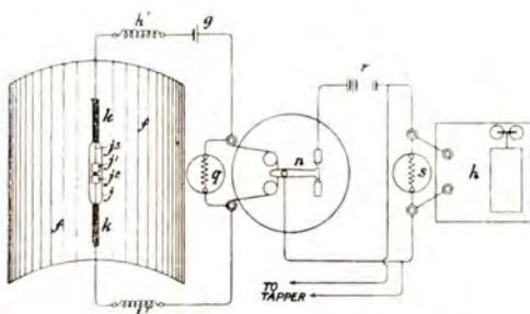
FIG. 2.—Coherer Receiver and Sheet Metal Reflector, 1896.
