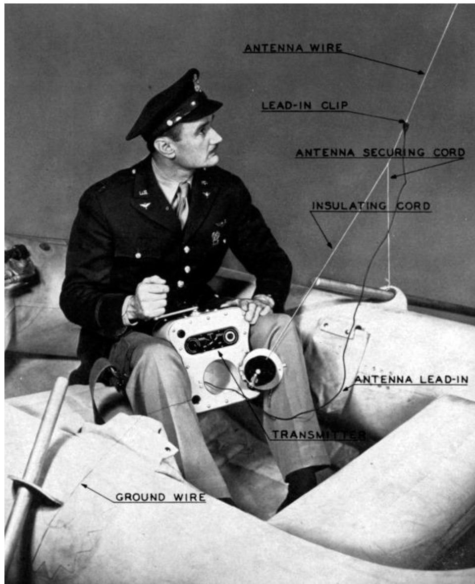
A manual excerpt shows how the BC-778 Transmitter is held between the legs and cranked for a charge.
