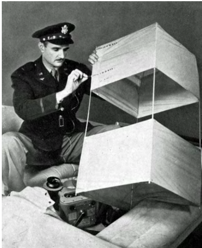
A manual excerpt shows the BC-778's spooled wire being connected to the M-357 box kite.
