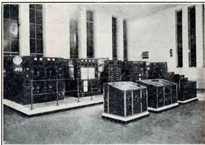
Marconi Short-Wave Transmitter at the League of Nations Wireless Station. Switch gear permits use of any of four waves selected between 14 and 100 metres.
