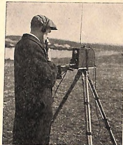
Fig. 3—Complete "Transceiver" equipment mounted on tripod for field service.
