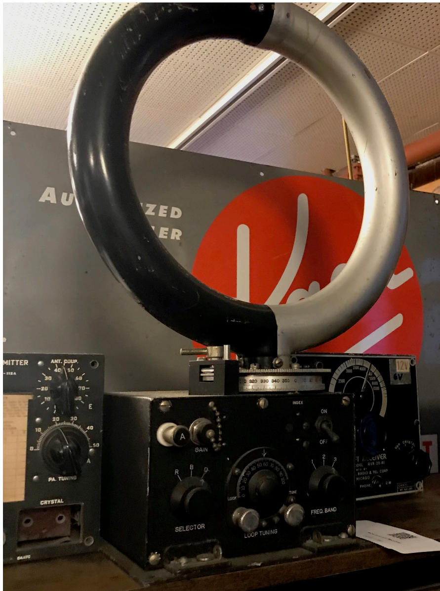
The Bendix Loop Antenna system (donated by Steve Keachie, x U/C labs) in the US Navy version, model DU-1.
