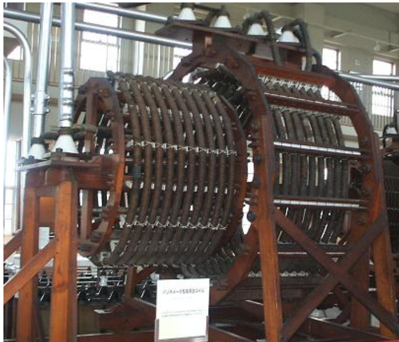
A Tuning Variometer for the Alternators.
