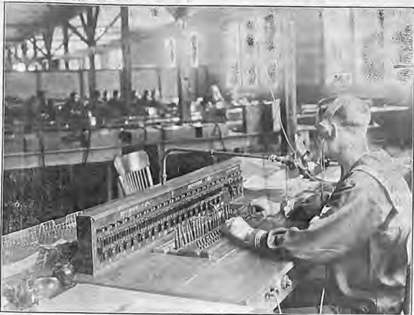
This switchboard, constructed at the school, enables phone communication over the radio practice circuits. Its possibilities offer a remarkable field for study. Snapped at the Commons.
