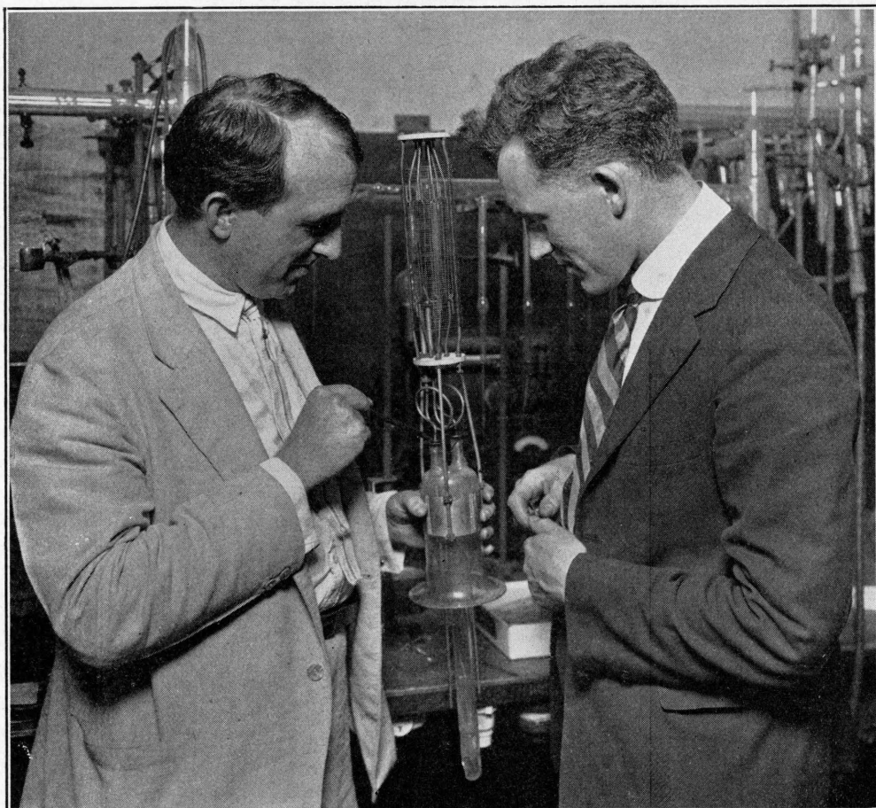
THE INTERNAL ASSEMBLY OF THE 100 K. W. WATER COOLED TUBE
