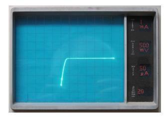
As a comparison, the last plot shows the response of a 1N56 germanium detector, at least 60 years old. Here, the conduction starts abruptly at about 0.25 volt. The 1N56 is a high-conductivity version of the venerable 1N34 germanium diode.
