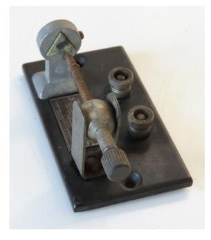
The detector operates by presenting a non-linear conduction curve to the RF impressed across it. The non-linearity translates variations in the amplitude of the RF wave to a signal that is presented to headphones connected to the detector.
