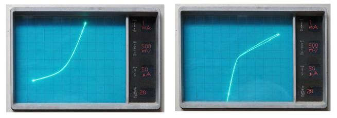
The first plot shows a gentle non-linearity with maximum curvature at a voltage of about -0.5 volts across the detector. At more negative voltage across the detector, the current decreases, and with positive potential, the current continues to rise. Thus, the resistance varies with the voltage across the detector. The detector in this mode would work best with a bias of 0.5 volts across it.
