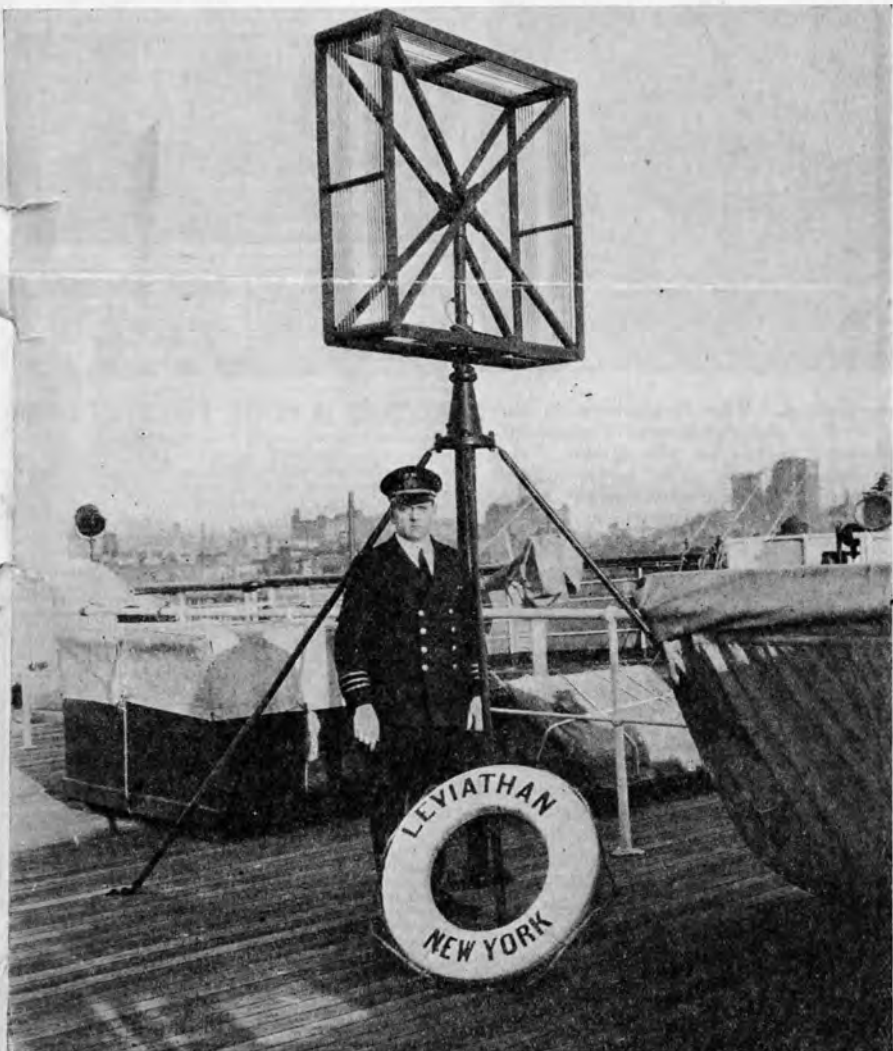
The five-wire cage which is part of the antenna equipment of the Leviathan's broadcasting station
