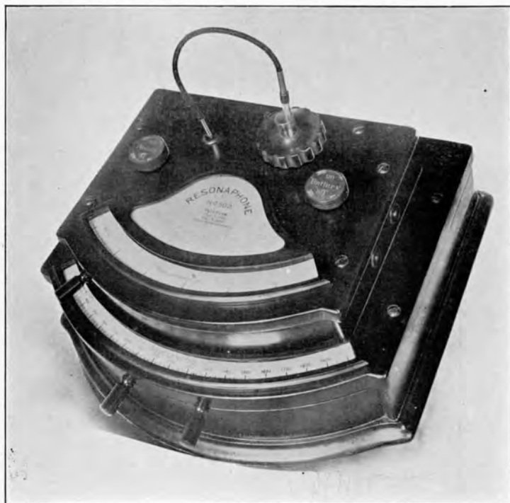
FIG. 13.—DETECTOR MOUNTED ON WAVE METER.
