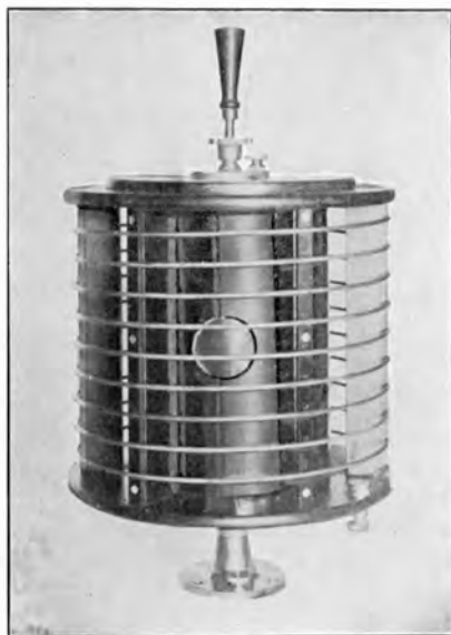
FIG. 6.—SPARK-GAP WITH MUFFLER, SURROUNDED BY INDUCTANCE.
